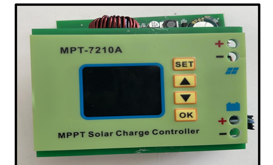
Figure 3: MPT 7210A Solar Charge Controller
